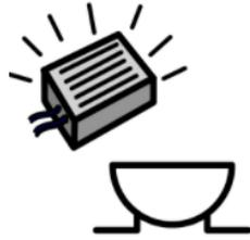
Buzzer: an automatic signalling device. They are used as alarms and door bells.
